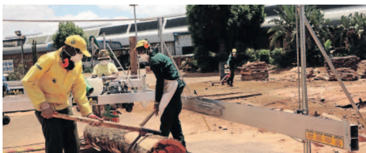
Workers prepare the wood from a blue gum tree to be cut to cants and further processed into planks.
