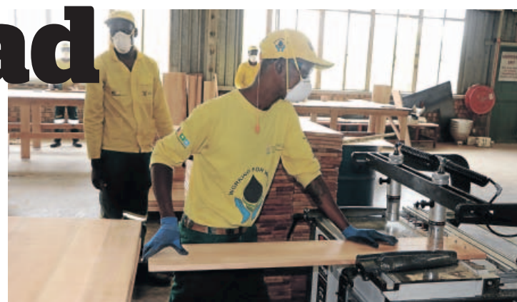
The planks are being smoothed around the edges using the edge sander.
