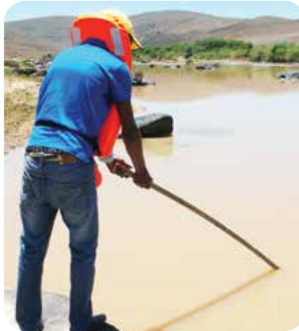
Above: A citizen technician taking a suspended sediment sample using a pole and jar sampler.
