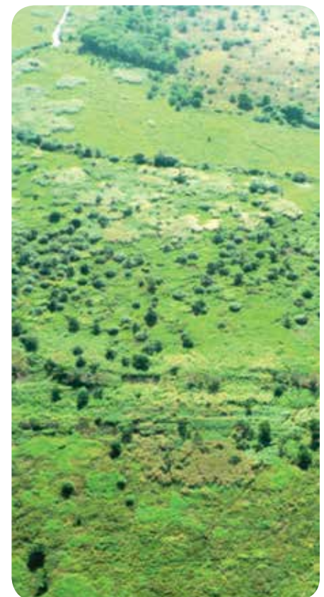
Above: Some of the earth berms (back ground) dissecting the Kleinspan interrupting natural flow patterns, whilst removed berms and associated revegetation are evident in the foreground.
