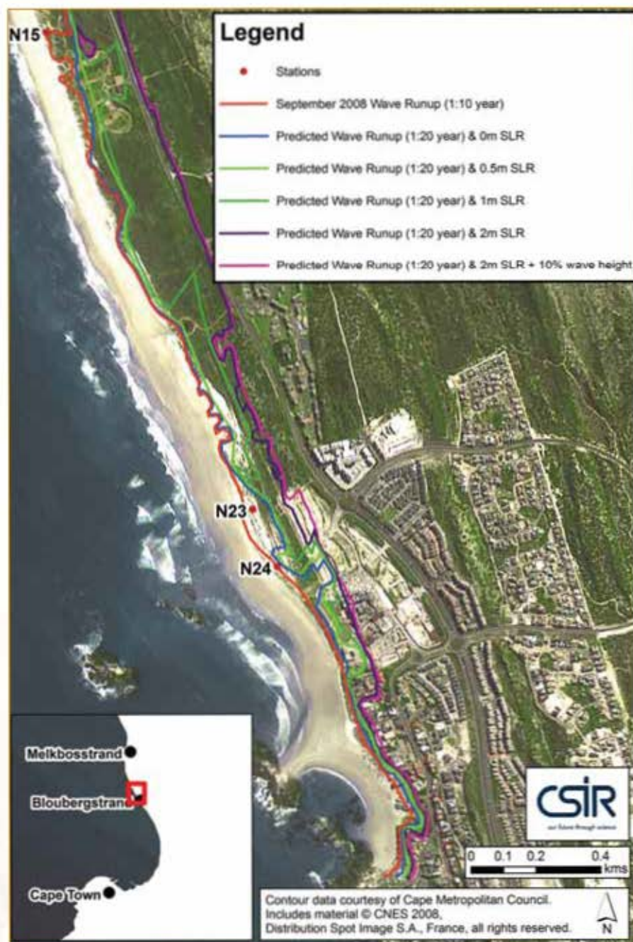
Map 8.5. Illustration of predicted effects of climate change on coastal runup lines near Blaauberg. Source: Theron, Diedericks, Maherry and Rossouw, CSIR (2010).
