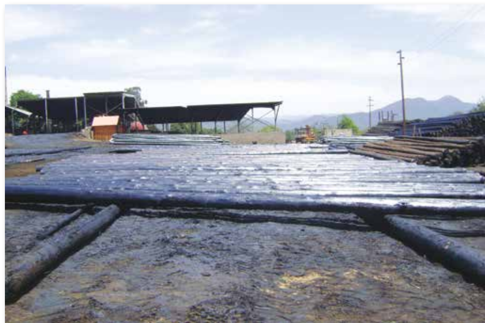
Processing area: Contaminated soil due to it being unlined
