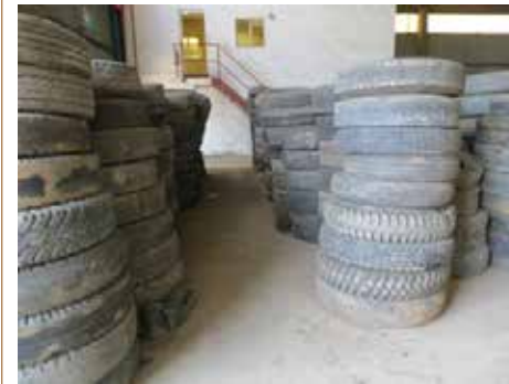
Photograph 3: Inadequate firebreaks between tyre stockpiles.
