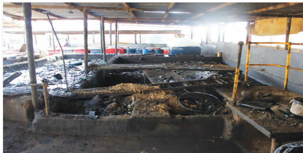
The area where used oil are poured into to facilitate water and oil separation
