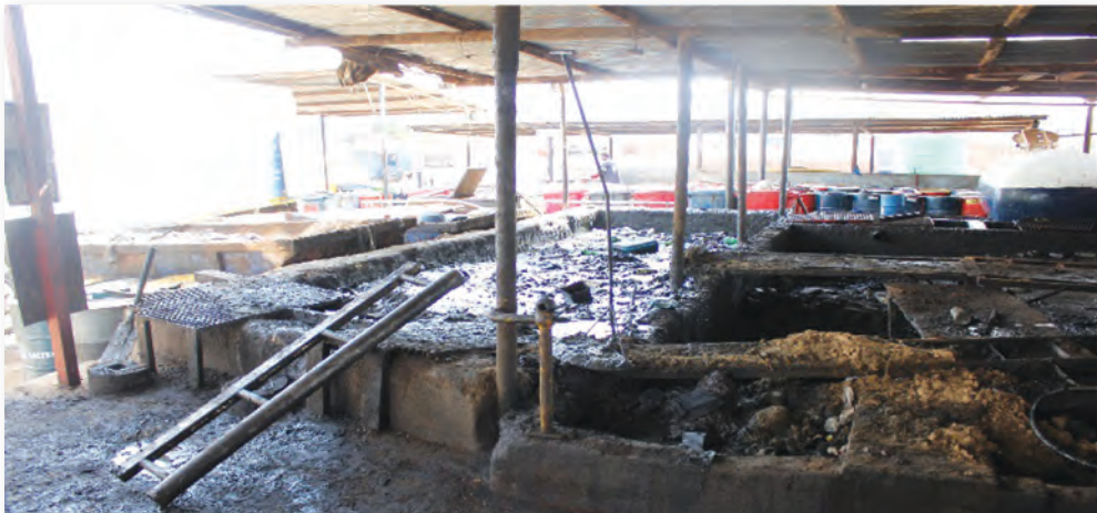
27:Oil/sludge separation process in the pond
